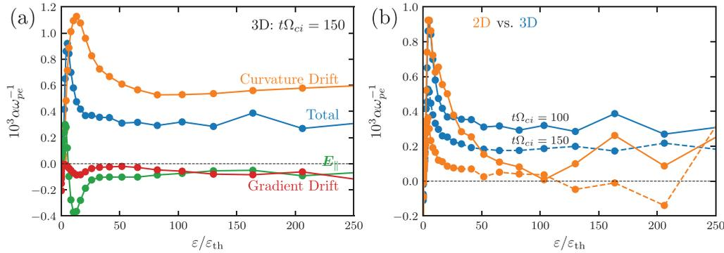
**FIG. 7.** Energy-dependent electron acceleration rate  $\alpha$ : (a) the contributions to  $\alpha$  by the acceleration associated with curvature drift, gradient drift, and the parallel electric field in a 3D simulation. (b)  $\alpha$  for the 2D (orange) and 3D (blue) simulations at two time slices. Reproduced with permission from Li *et al.*, *Astrophys. J.* **884**, 118 (2019). Copyright 2019 Institute of Physics (IOP).
